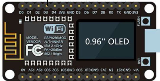
module esp8266 + 0.96" OLED
